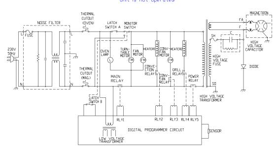
SCHEMATIC DIAGRAM NDTE: Door is closed Unit is not operated
