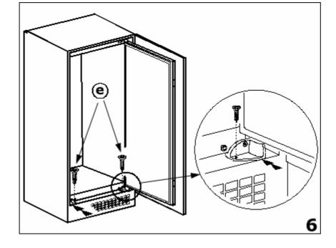
**6)** Align the front feet of the appliance, with the front edge of the kitchen unit.
