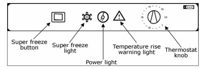
You switch on your appliance by connecting it to your mains supply and setting the thermostat. The thermostat is located on the control panel, at the top of the freezer.
