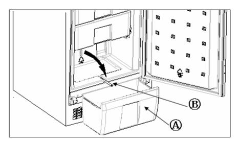
Your appliance is fitted with a defrost drainage tube. Therefore you should pull out the bottom drawer (A) and place it on the floor in front of the appliance.
