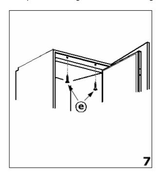
**7)** Screw the top fixing bar to the underneath of the kitchen unit using the  $\emptyset 4 \times 17$  fixing screws (**e**).
