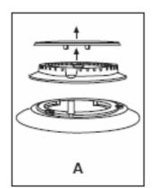
Remove the pan-stands, burners and flame spreaders (A).
