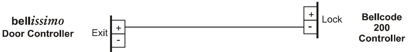
Connect the lock release as per this manual. Leave the Bellcode controller set to fail secure, the BSD controller sets the lock type.
