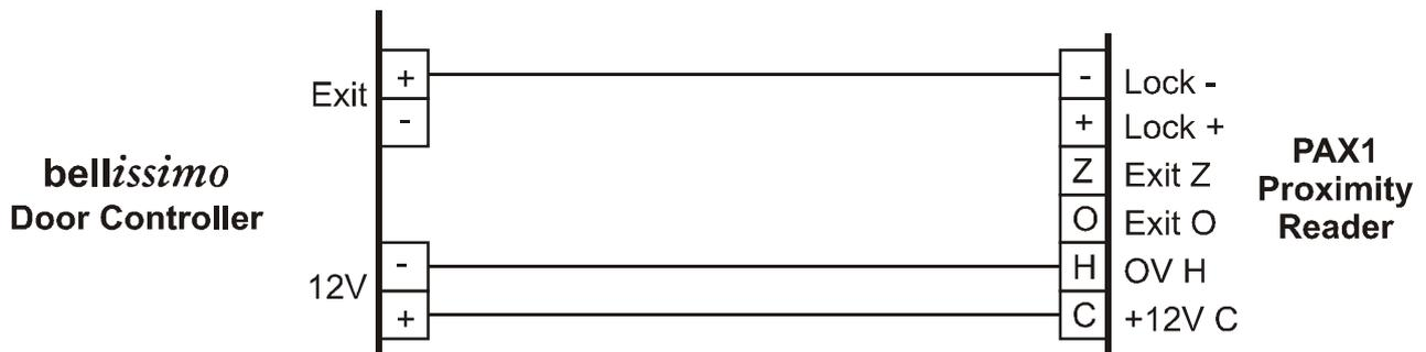
Connect the lock release as per this manual. Leave the Proximity Reader set to fail secure, the BSD controller sets the lock type.
