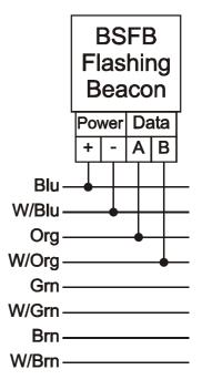
Option 2: Locally powered from separate PSU
