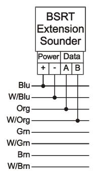
Option 2: Locally powered from separate PSU
