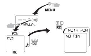
If a PIN code has been activated, the timer can no longer be activated without a valid PIN code after a RESET.
