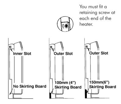
Note that the smallest wall spacing should be used only when the skirting board is of the modern slim type, or there is no skirting board at all. THE HEATER MUST STAND VERTICAL
