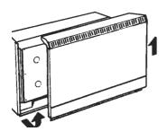
remove the screws fixing the rear flange of the top panel, and remove the two screws along the bottom edge of the front panel. Carefully swing out bottom of front panel and lift assembly clear of casing, this operation also removes the control knobs under the flap. Put assembly in a safe place to avoid damage to paint etc.
