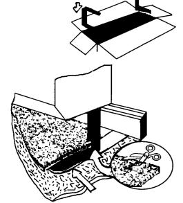
It is preferable to fit the heater feet whilst the heater is still in its carton. Turn the carton upside down and open the bottom flaps. The corner fitments contain both feet and the fixing kit.
