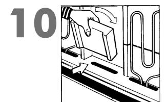
Put in place the rear rank of bricks, pushing them well back against the rear insulation. Replace the element, making sure that the connection is tight.
