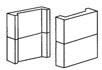
Note the way the bricks are positioned in the heater. Otherwise they will not fit.
