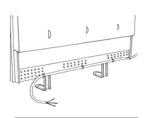
When bracket is securely fixed, replace the heater under the bracket angle and align screw holes on heaters ends. There are two fixing slots at each end of heater, allowing different stand-offs for different thicknesses of skirting board. Do not fully tighten these screws until the bricks are loaded into the heater as some settling of the heater may occur.
