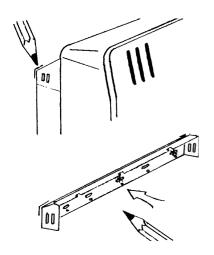
If mains connection is to be made from the left hand side, at this point the mains lead must be secured to the back of the heater using ties provided in the fixing kit.
