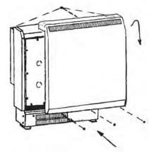
Take care not to trap wires or the thermostat capillary between the panel flanges. Ensure all washers are replaced in their original positions.
