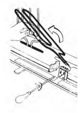
Note the way the bricks are positioned in the heater. Otherwise they will not fit.
