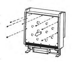
Temporarily remove one central element to provide access for the rear rank of bricks.
