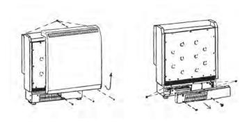
The top panel and front panel are joined and should be removed as one assembly. To do this, remove the screws fixing the rear flange of the top panel, and remove the screws along the bottom edge of the front panel. Carefully swing out bottom of front panel and lift assembly clear of casing, this operation also removes the control knobs under the flap. Put assembly in a safe place to avoid damage to paint etc.
