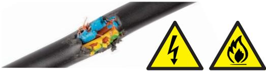
Frayed or split insulation on power cables give a leakage point for current to electrocute. At worst a shock of 240v can be fatal. A similar risk occurs if cables are pulled to strain or loosen a termination point, to leave either an exposed 'live' conductor or broken conductor strands.
