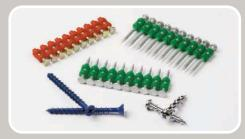
Most plastic wall-plugs will soften and fail later, disintegrating between 100°C - 200°C, so provide inadequate support in fire conditions for the time required. We recommend fire-rated fixings such as the DeWalt® Wall-Dog®. Simply drill a 4mm pilot-hole in the substrate, through the PVC trunking if applicable, insert the Safe-D® Clip and the Wall-Dog. Sharp flutes along the shaft negate the need for plastic wall plugs. Wall-Dogs are EN certified as 2 hour fire-rated.
