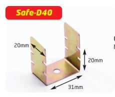
Can fit 32-40mm trunking bases folds to max 20mm height
