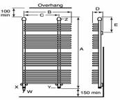
W = electrical element cable termination X = water inlet (flow) connection Y = water outlet (return) connection Z = bleed valve
