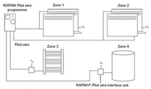
Note: Pilot wire installations are appropriate for single phase connection only.
