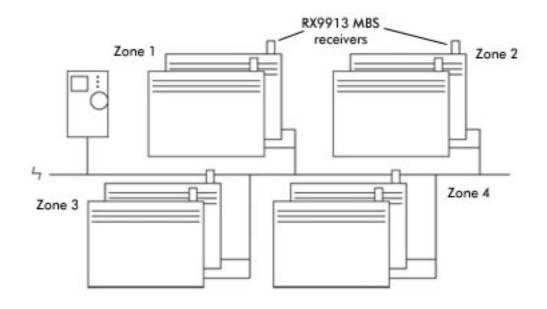
Note: Heaters and programmers should be installed on the same supply circuit, connected to the same phase. For a 3ph installation a phase coupler should be used.
