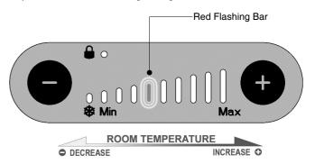
After 10 seconds the temperature control display will return to the **Comfort Heat** control mode.
