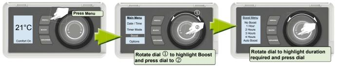
Auto Boost will automatically use the boost element to maintain the set temperature during '**Comfort On**' periods. Note: Boost element uses peak rate electricity and this could lead to increased running costs.
