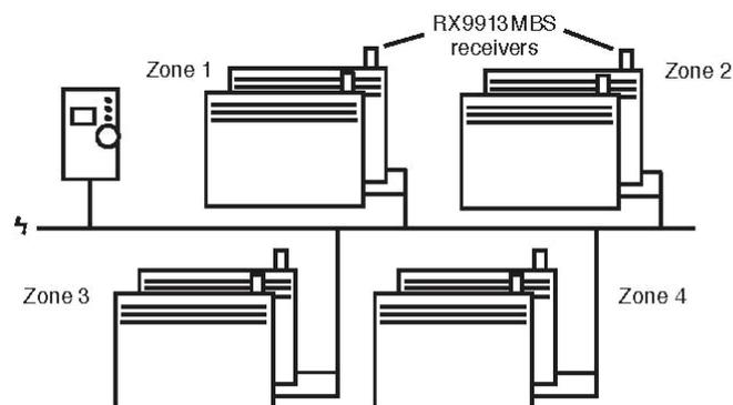
Note: Heaters and programmers should be installed on the same supply circuit, connected to the same phase. For a 3ph installation a phase coupler should be used
