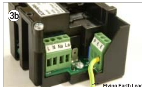
3b. The cables should be connected to the terminal blocks on the unit as follows:
