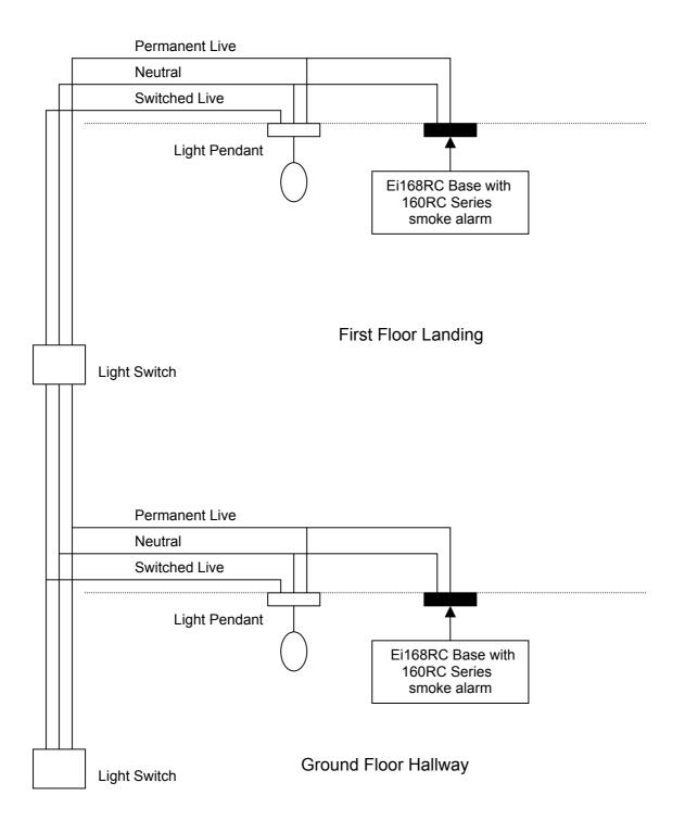
NOTE 1: The circuit shown is an example only. The only important part is that there MUST be a permanent live and neutral connection to the smoke alarms from the light pendant
