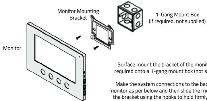
Surface mount the bracket of the monitor or if required onto a 1-gang mount box (not supplied).
