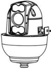
3. Remove cover to access address/ baud rate/resistor switches (see page 5)
