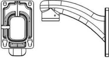
1. Mark out the holes for the 4 fixing screws using template provided
