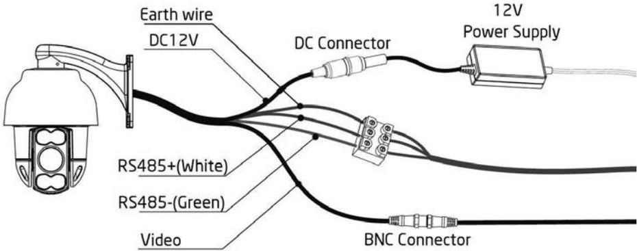
**Using a screened control cable is recommended for maximum protection against interference.**
