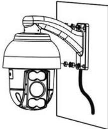
7. Insert fixing screws and secure bracket to wall
