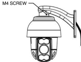
6. Insert M4 screws into bracket to secure dome housing
