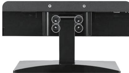
1. Before mounting the monitor, remove the base riser (vertical portion of the base) by removing the two screws at the top with a screwdriver. Then the base and the riser can be removed. In order to prevent losing the two screws, we suggest replacing the screws in their original holes.
