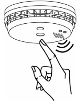
Figure 6: Testing the Smoke Alarm
