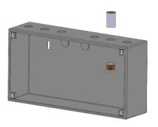
A harness is provided that extends from the battery box to the control panel. Connections are described below. You must run the harness through the knockout (removed above), through the coupling and up to the control panel battery terminal (BAT+ BAT-)
