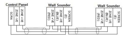
MAGDUO Wall Sounders can be mixed on the same zone as other types of MAGDUO device. The above diagram shows how to make the zone positive, zone negative and screen connections between the control panel and MAGDUO Wall Sounder. Refer to the instruction leaflets supplied with other MAGDUO devices for their equivalent wiring/terminal labelling details.
