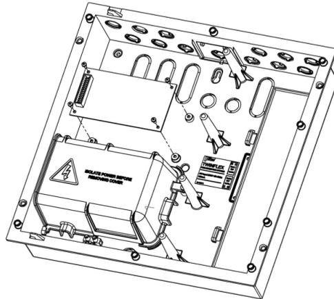
7. Plug one end of the ribbon cable assembly into the expansion card PCB (this will only fit one way).
