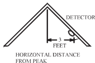
Figure 5: Recommended location to mount smoke and heat detectors in rooms with sloped, gabled, or peaked ceiling
