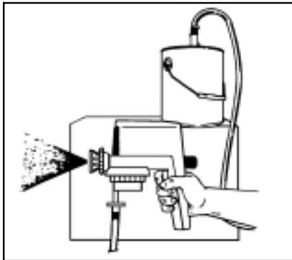
**WARNING-** The filter must be completely submerged in the paint at all times. If not completely submerged and air is sucked into the system, the piston could seize. If the piston seizes, the sound the gun makes will change to a low hum and the gun will quickly become hot. Stop using immediately. Clean and lubricate gun thoroughly before re-using.
