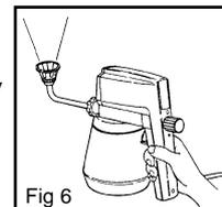
easier. As the sprayer must not be tilted at more than a 45° angle to prevent a back leak, it is essential to use the flexible extension to paint ceilings (fig 6).
