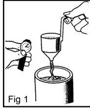
Follow the manufacturers guide for thinning inconjunction with a spray gun. If in doubt please consult the manufacturer of the paint. The viscosity cup supplied will help you determine the correct thickness of the paint.
