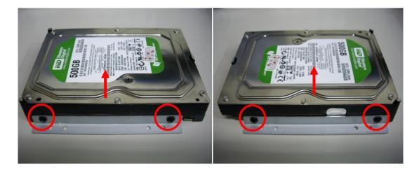
Step 2) Place the HDD on the HDD plate and screw it as indicated.
