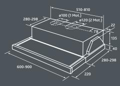
Finish White with stainless steel front panel 3 speed slider control Controls Lights 2 x 40w hob lamps Grease filter Metal washable grease filters **Ducting connector** 125mm (5in) diameter ducting connector Available widths 600mm or 900mm Maximum airflow 480 m<sup>3</sup>/h IEC airflow 430 m<sup>3</sup>/h
