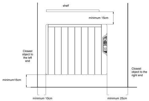
Position and fix the brackets at the correct distance from the floor and hang the unit on the hooks of the brackets. And mark the wall. Use the polystyrene packaging to level the heater and protect the floor
