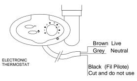
Connect the black wire marked "FIL PILOTE" to the signal wire when available. (Not available in UK).
