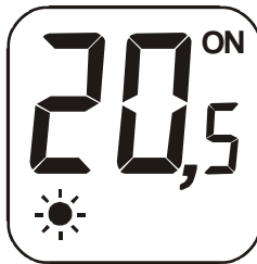
Example of the heater permanent COMFORT mode, Set point temperature is 20.5°C, showing ON output condition.
