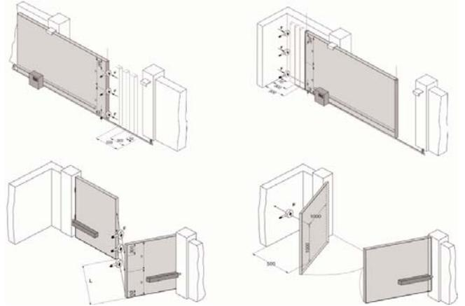
Figure 3 – measurement points for force testing to EN 12445
