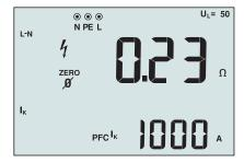
Figure 13. Line Impedance Display
