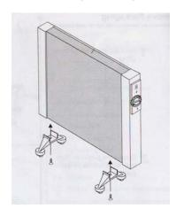
Check the stability of the heater by standing it on a flat level surface
