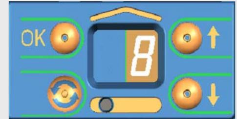
2) Bring the controller into radio link creation mode, the LED lights up orange
