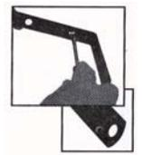
*Once a suitable location has been selected, fix the bracket securely.*
