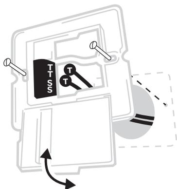
**C)** Attach the thermostat to the wallplate when finished.
