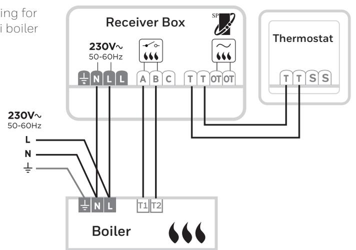
C) Wiring for OpenTherm boiler
