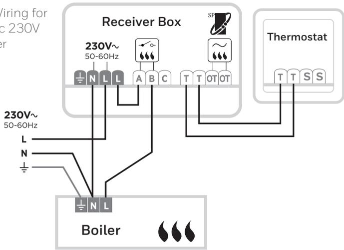
B) Wiring for Combi boiler
