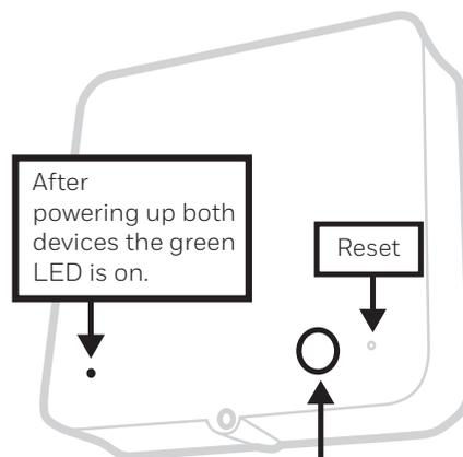
After powering up both devices the green LED is on.
