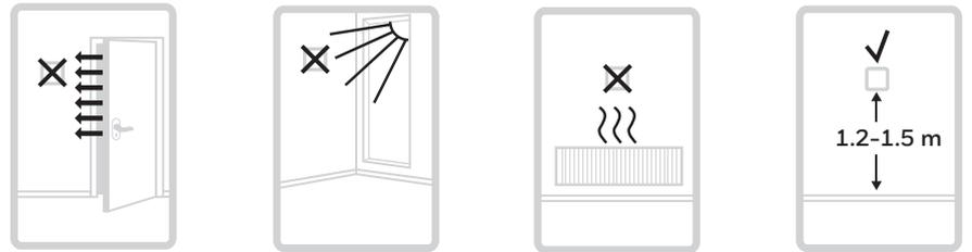
The T6 thermostat should not be placed near draughts, in direct sunlight or near heat sources. It should be at least 1.2 - 1.5 meters from the floor.
