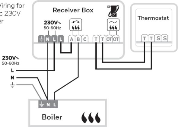
B) Wiring for Combi boiler
