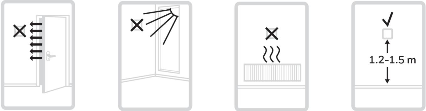
The Lyric T6 thermostat should not be placed near draughts, in direct sunlight or near heat sources. It should be at least 1.2 - 1.5 meters from the floor.
