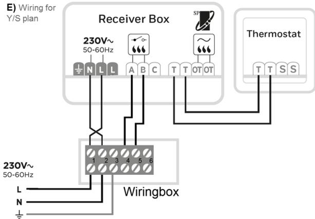
Note: Wiring diagrams are for Lyric T6 wired thermostat solution, for Lyric T6R wireless thermostat the thermostat is not wired to the Receiver box and the terminals are also not available.
