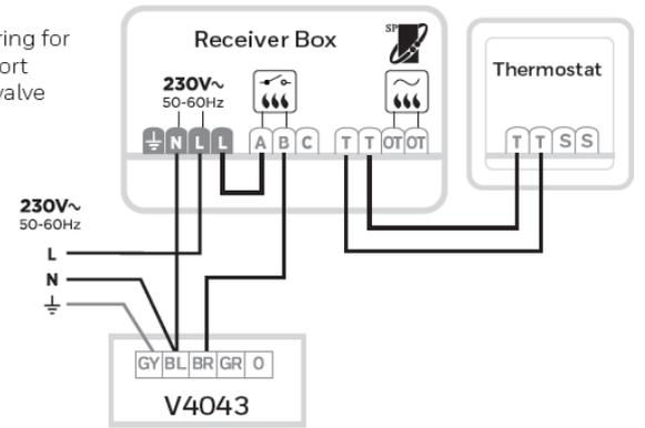
E) Wiring for Y/S plan
