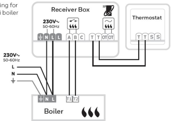
C) Wiring for OpenTherm boiler
