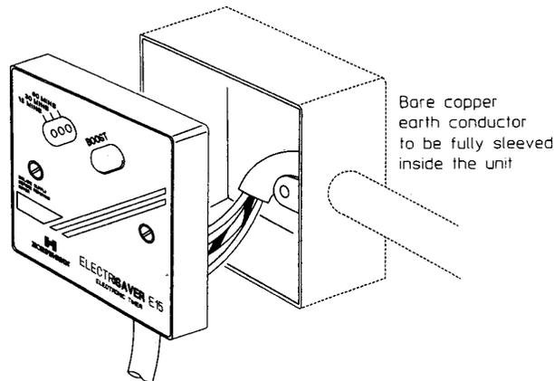
Use twin and earth cable with a minimum conductor size of 2.5mm<sup>2</sup> to connect the Electrisaver to the supply. Use a suitably rated three-core flexible cord (see below) to connect the Electrisaver to the appliance to be switched.
