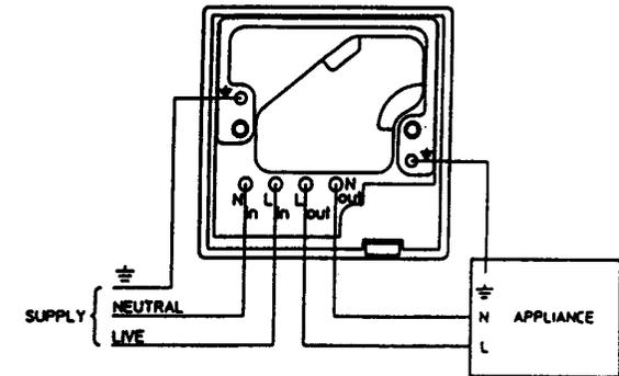
Remove cut-outs before fixing the box. Where appropriate drill the box to provide close fitting entry for cables and heat-resistant flexible cords. Take care to remove sharp edges. All un-insulated earth conductors must be sleeved and connected to the earth terminals on the back of the Electrisaver.
