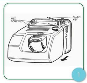
Position the dryer as shown in the diagram Release the casing from the back plate by removing the two hex screws with allen key.
