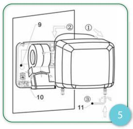
Replace the casing and secure the hex keys with the allen key.
