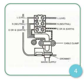
Release the cable clamp. Pierce the grommet cap (supplied with the screws and plugs) and slide it over the cable end. Bring the mains supply cable through the grommet and connect the mains supply cable to the terminal block on the fitting, using the following colour code for the wiring:
