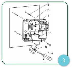
Using the template (back page) mark the positions for the fixing holes. If the mains supply is to be concealed, drill out the cable entry hole. It is important to ensure the template is level when marking the positions on the mounting surface.
