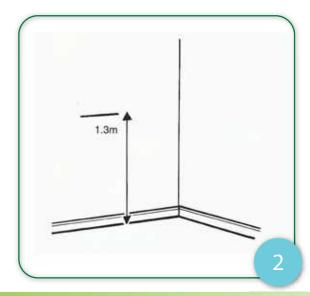
Position the dryer as shown in the diagram. Please Note: For new installations, check for any electrical
