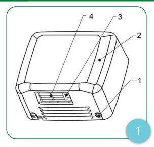
Remove the hexagonal drive screws from the base of the dryer using the key supplied.
