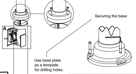
Class II Wiring. Mains supply in Base. Double Insulated - No Earth Required.
