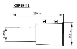
Max pole diameter to insert into the fitting aperture -KSR99110 & KSR99111 would be Ø60mm - Accessory KSR99116 reducing spigot to fit a Ø76mm - Pole -**Tighten to 16NM**
