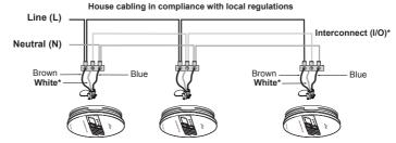
NOTE: Use standard British Standard household cable PVC/PVC 6242Y / 6243Y or equivalent in accordance with local regulations.
