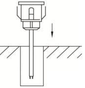
**2.**Feed the pre-installed 2 metre cable through the hole and make any electrical connections which may not be accessible once the fitting is totally installed.
