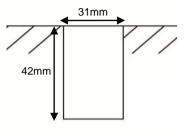
**1.**Mark the position(s) of where the fittings are to be installed ensuring not to infringe with any joists, gas, water pipes or electrical cables that may be hidden below the surface. Using a suitable hole saw cut a hole approximately 31mm in diameter & 41 mm deep
