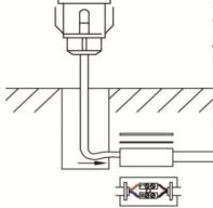
**3.**Connect the preinstalled flexible cable to a suitable joint box ensuring correct polarity is observed. BROWN- LIVE. BLUE-NEUTRAL. The joint box must be IP65 or above rated if used externally.
