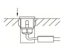
**4.**Select one of the 3 supplied bezels and screw it onto the top of the fitting the stainless steel bezel is pre-fitted, must be removed before installation of one of the chrome accessories
