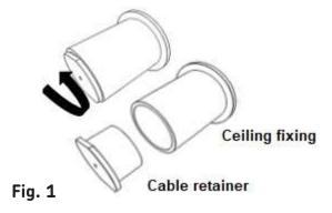
• Fix the ceiling fixings to the ceiling using suitable screws and plugs (not included). The fixings should be the same distance apart as the holes in the luminaire (see Fig. 2)
