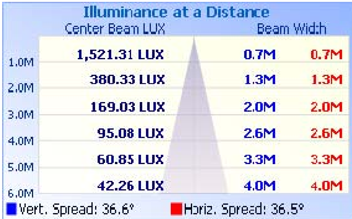
Figure 5. Illuminance cone diagram.
