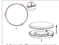
3. Remove the diffuser screws and separate it from the base.
