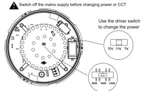
Use the LED gear tray switch to change the CCT temperature
